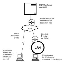
This means users will be able to connect their PCs directly to the DLSw router next to the SNA host, using only an existing standard TCP/IP router at the remote location. As the diagram at right shows, this technology – called Desktop DLSw– gives MIS an extremely flexible, TCP/IP-based networking implementation. It maintains the integrity and functionality of native SNA, but it can be deployed in a variety of environments where router-based DLSw is not practical.
