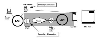
Users may use an SNA gateway as a default connection in a parallel backbone network. Should the gateway connection become unavailable, resuming a true SNA connection is as easy as opening a new session with the Desktop DLSw connection. This connection takes place across a native SNA connection using the parallel backbone router network.
