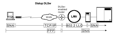
Desktop DLSw is a ubiquitous solution which allows users to dial up asynchronously into an IBM mainframe or midrange computer with no intermediate gateway. The client software uses the same technology as it does when connecting to the Internet or a remote LAN.
